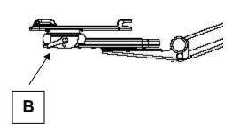
Height Adjustment: There are no levers needed to adjust the height of the keyboard tray. To raise the tray, lift it to the position you want. To lower the tray, tilt the front of the keyboard tray upwards and lower the tray to the position you want.
