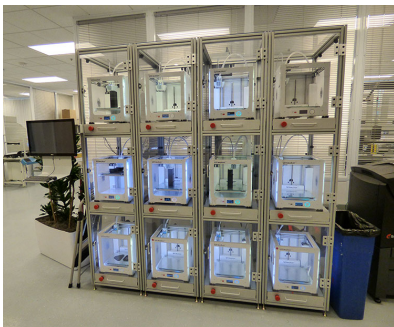
Example of exhausted enclosure.
