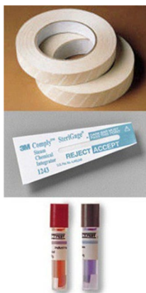
Figure 8-6: Devices to indicate proper function of an autoclave
