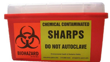
Figure 8-3: Sharps container for chemical contaminated sharps
