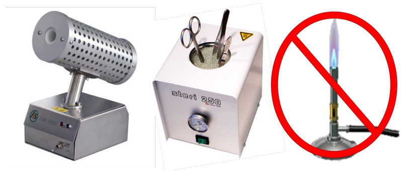
Figure 4.4 Alternatives to use of flames inside a biosafety cabinet
