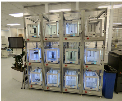
Example of exhausted enclosure.
