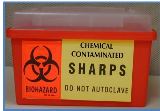
Figure 8-6: Sharps container for chemical contaminated sharps.
