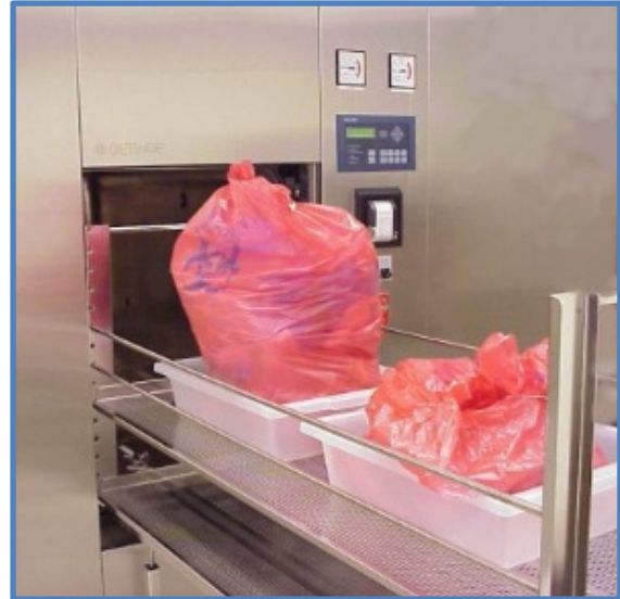
Figure 8-14: Biohazard bags placed in autoclavable secondary containers prior to autoclaving.
